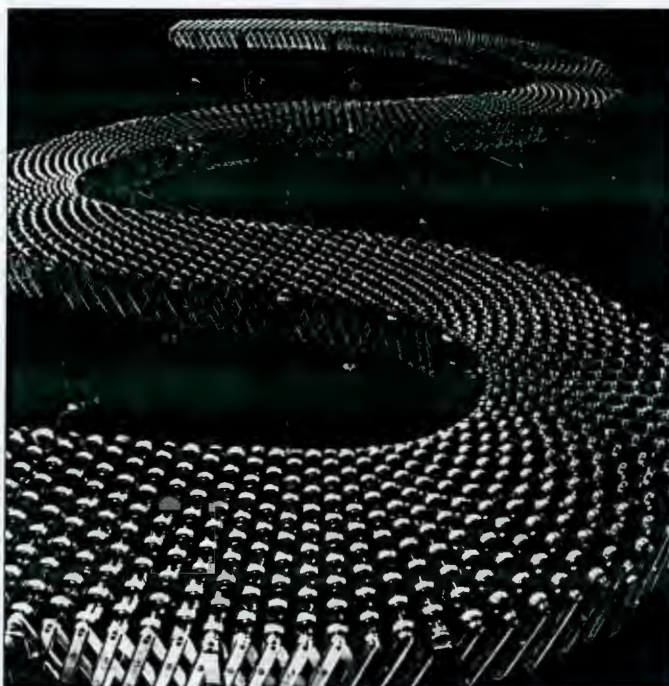
BEST conveyors are portable, expandable and extremely flexible. Packages are self tracking which means they follow the conveyor path without side rails or engineered curves.
