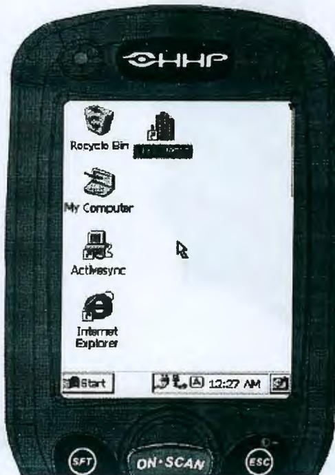
Use the cursor keys to navigate around the screen. For a left mouse click, press either one of the ENT keys. Use a left mouse click to select an item or launch a program. For a right mouse click, use the TAB key. When you use a right mouse click, a menu of items pops up and tells you what actions you can perform, and shows you shortcuts. To open files or applications with a double click, tap the ENT key twice in rapid succession.
