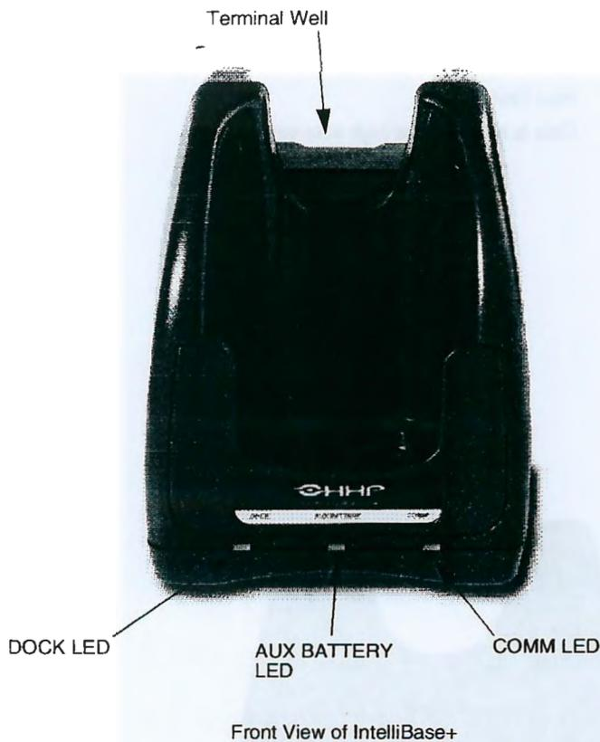
**Dolphin Terminal Well** Place the Dolphin in this well to communicate with a host device and to charge the Dolphin's battery.
