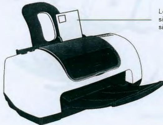
Load the printable side up and the flap side down.
