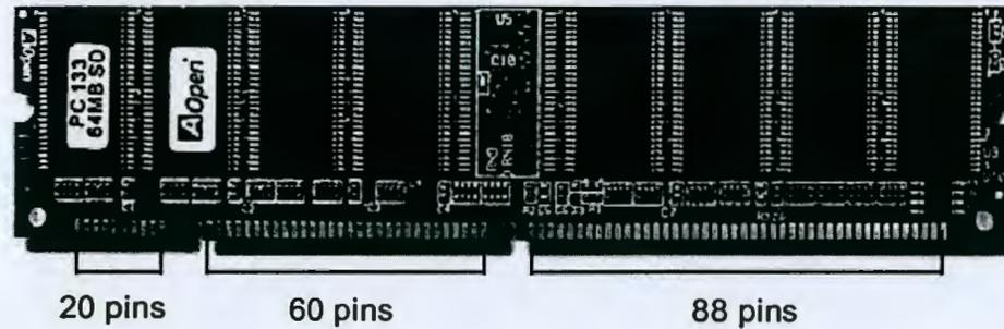
2. Insert the module straight down to the DIMM slot with both hands and press down firmly until the DIMM module is securely in place.
