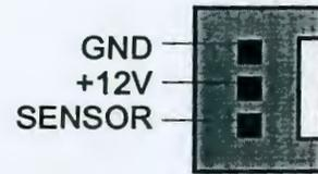
**Note:** Some CPU fans do not have sensor pins; therefore, they cannot support fan monitoring.
