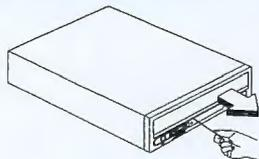
1. Locate the tiny hole at the bottom of the disc tray. Gently poke the hole three times with a sharp needle or a clip.
