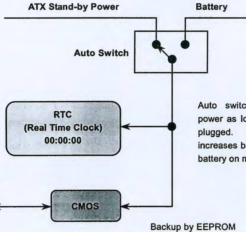
Auto switching to ATX standby power as long as AC power line is plugged. This smart design increases battery life if you still plug battery on motherboard.
