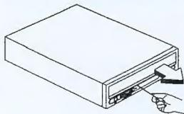
1. Locate the tiny hole at the bottom of the disc tray. Gently poke the hole three times with a sharp needle or a clip.
