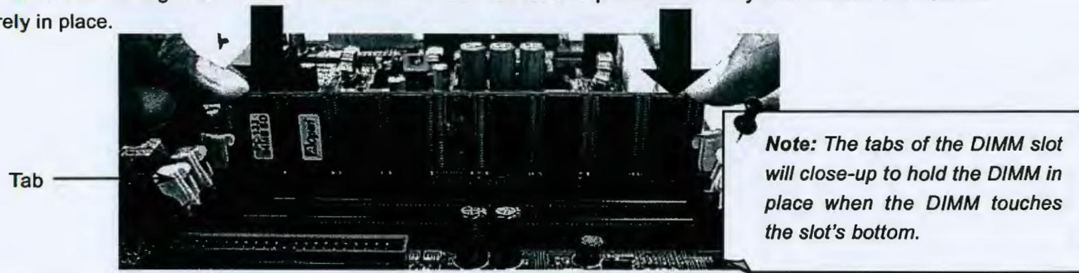
3. Repeat step 2 to finish additional DIMM modules installation.
