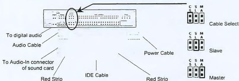
**NOTE:** The red edge of the IDE cable corresponds to pin 1 of the IDE interface on the CD-ROM drive.
