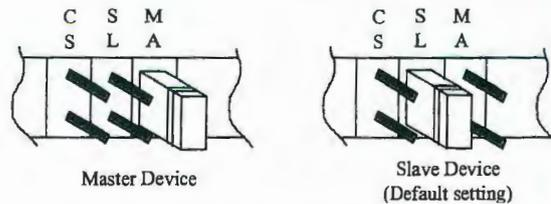
Figure 2: The setting of Master or Slave device.
