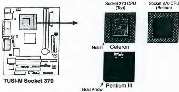
1. Locate the Socket 370 and open it by pulling the lever gently sideways away from the socket. Then lift the lever upwards. The socket lever must be fully opened (90 to 100 degrees).
