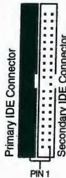
**NOTE:** Orient the red markings on the IDE ribbon cable to PIN 1
